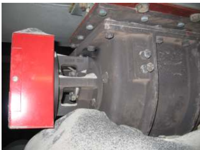
Rotary valve with leaking shaft seals
