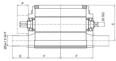
Tube diameter G can be made to suit. Tube length E can be made to suit. Standard rotor speed 20 rpm. Painted white gloss externally. Internally unpainted.
