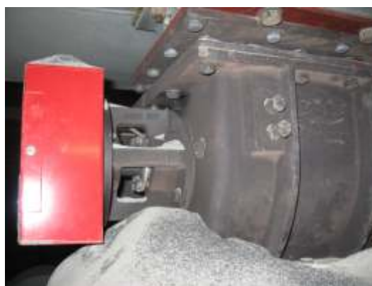
Rotary valve with leaking shaft seals
