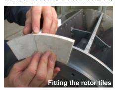
taking off the high spots naturally found when manually assembling the tiles.
